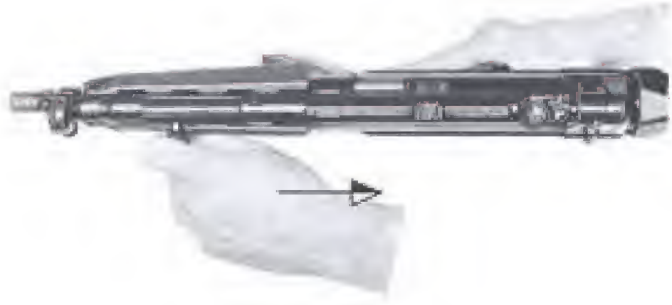
Fig. 26 Retracting the cocking lever
